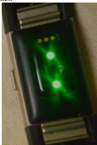
Figure 3: LED and photo diode sensor
