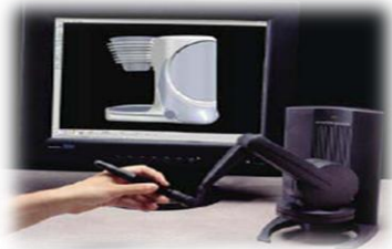
Fig: PHANTOM, which is a small robot arm with three joints each connected to a computer-controlled electrical DC motor.
